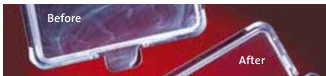
Blurry surface caused by dust
