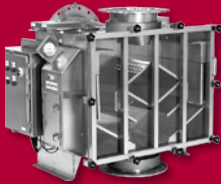
Max Series P400 to P2000 are equipped with double wash decks
